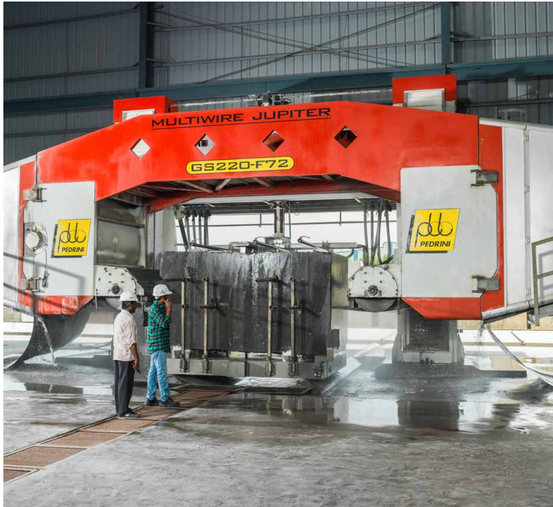
Multiwire Jupiter, Pedrini (Italy) 72 diamond wires, one pass, uniform slabs.
