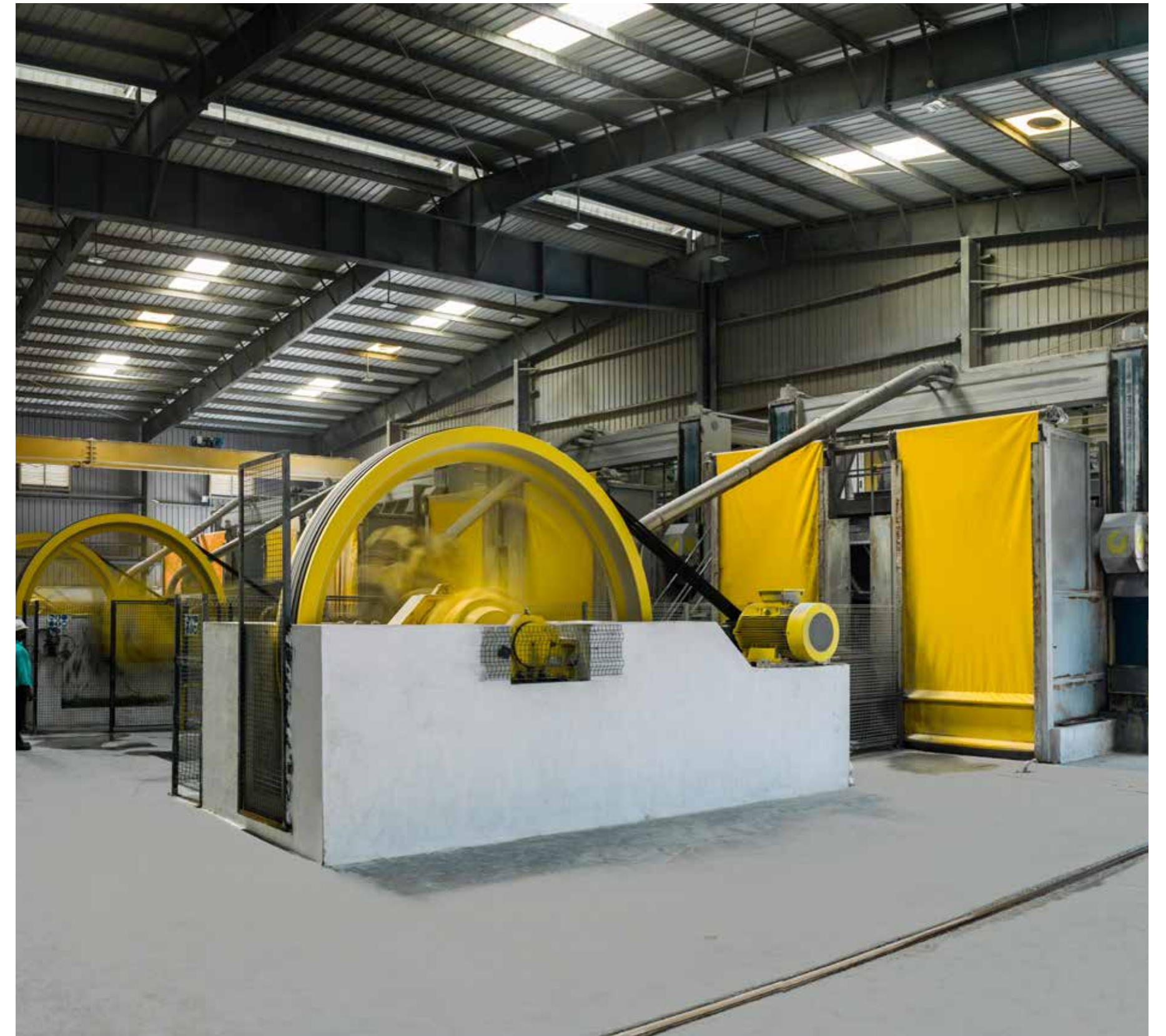
Gangsaw, Gaspari Menotti (Italy) 4.5 x 3.5 m frame, full-block precision cutting.
